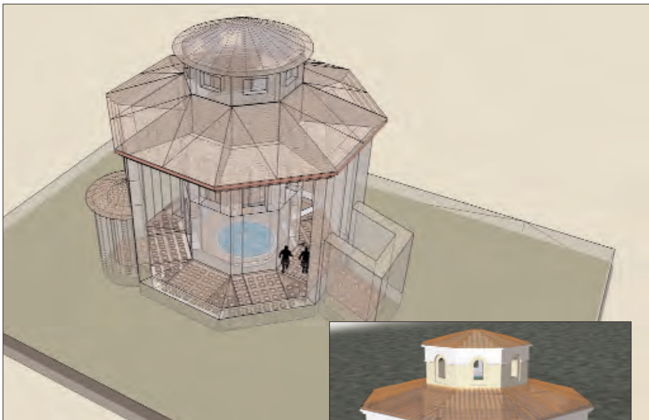
Fig.25. These computer models by Bartek Cichy all start with a virtual reality wire frame which has to be computed from the exact measurements obtained on site. Every surface has then to be filled with raster images and textures to recreate the
