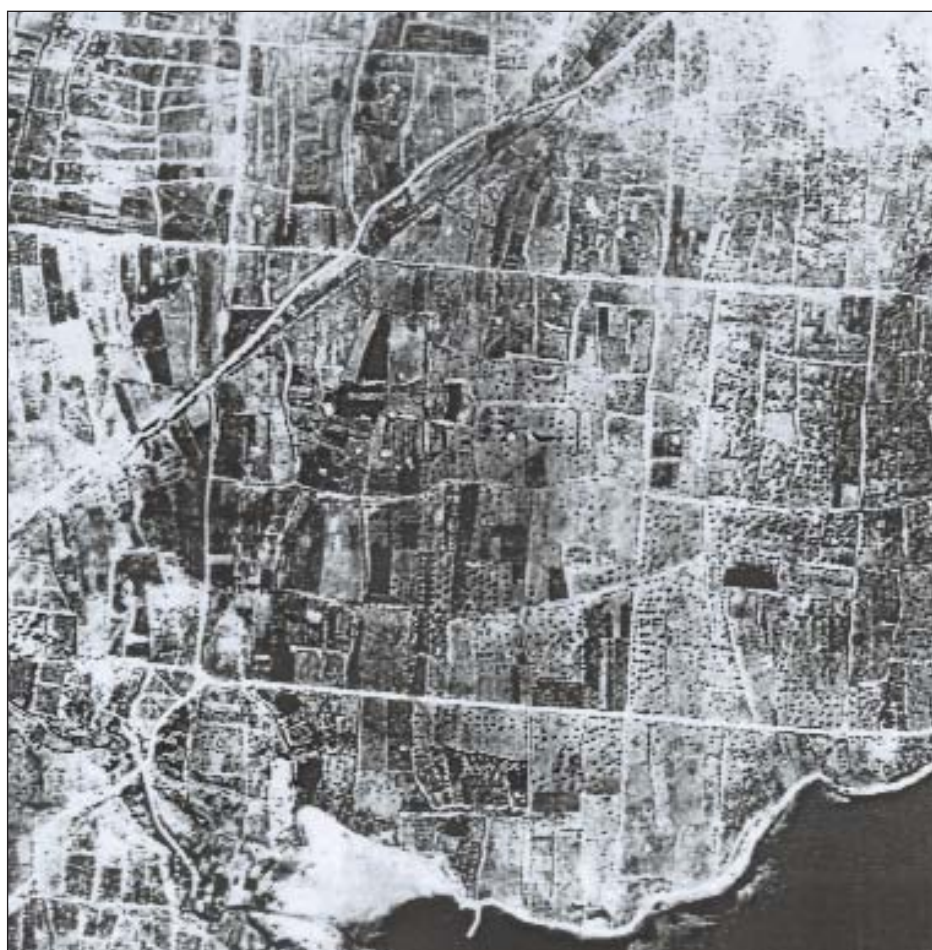
Fig. 36. Aerial photograph of the area around the town of Zadar in Croatia. The Roman land division in units of 20 x 20 actus still survives in a remarkable state of preservation. The normal size of a centuriae was a square of 20 x 20 actus measuring on one side 706m, with an internal area of about 124.6 acres (50.4 ha).
